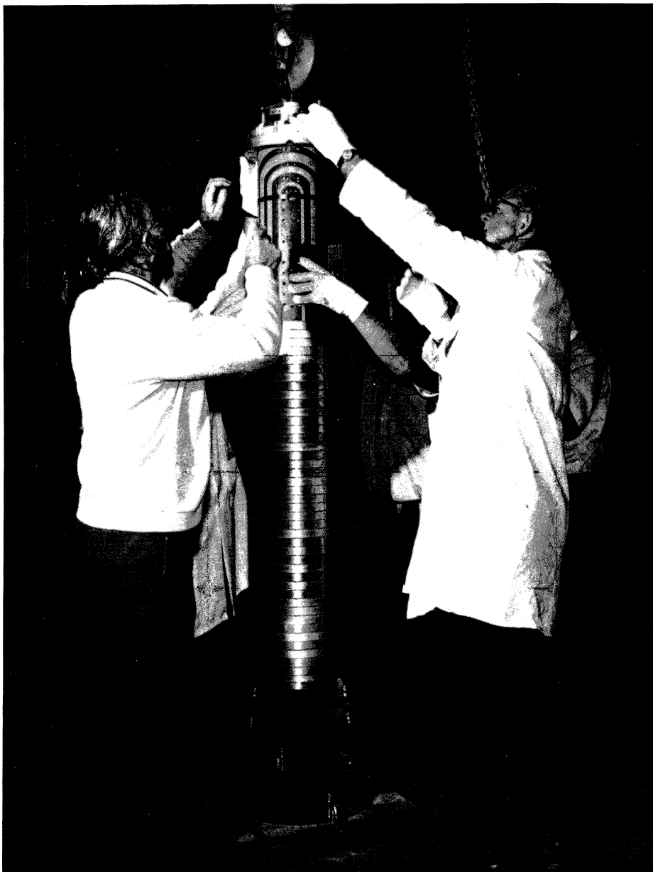
Last month we reported progress on the small superconducting accelerator/storage ring, ESCAR, being built at the Lawrence Berkeley Laboratory. The photograph shows one of the superconducting dipoles being assembled; its coil is being lowered into a stack of aluminium alloy rings. The conductor configuration can be seen on the half coil facing the camera.
